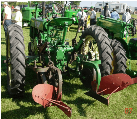
An early John Deere model B-3, 18-inch, integral two-way plow mounted on a vintage un-styled, John Deere model “B” tractor equipped with a “modern” hydraulic lift.
